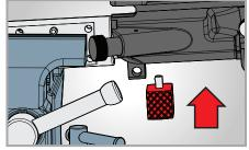
Lock Knob keeps the upper locked into the barrel lugs at any rotation
