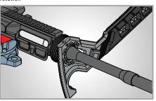
Steel barrel lugs absorbs the pressure of torquing barrel nuts and flash suppressors — not the upper housing
