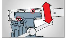
Vise Pins allow the upper to be positioned at different user-selected working angles and prevent unwanted rotation
